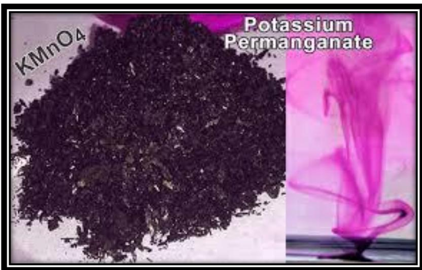
**Potassium permanganate is used extensively in the water treatment industry. It is used as a regeneration chemical to remove iron and hydrogen sulfide (rotten egg smell) from well water via a "Manganese Greensand" Filter. "Pot-Perm" is also obtainable at pool supply stores and is used additionally to treat waste water.**
